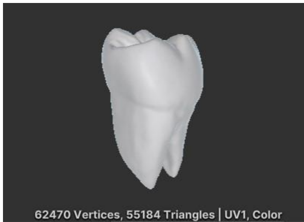
(a) Mesh representation of a tooth. Inside is hollow only surface is defined.
